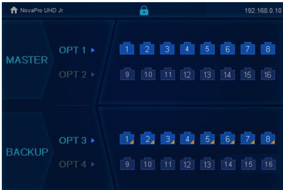
Figure 4-3 Optical fiber port statuses – Hot backup
